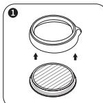
Push sealing disk through the attachment ring.
