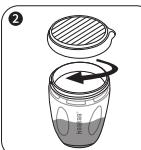
Screw the attachment ring onto the storage container.
