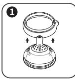
Push your chosen attachment through the attachment ring and into place. Ensure the bottom rim of the attachment is laying flat inside the ring.
