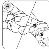
**DISASSEMBLY:** Use your thumb to pry up the bottom edge of the lid (see the arrows), then pull down the top edge of the attachment ring.
