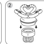
Once filled, press the Feeder lid tightly onto the attachment ring.
