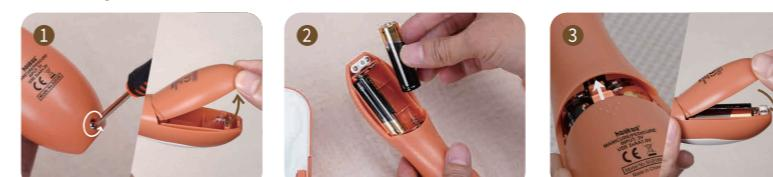
Use a Phillips head screwdriver to loosen the security screw. Remove the panel by sliding back then lifting.
